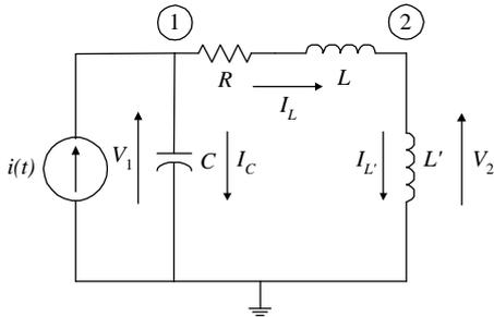
Fig. 6.1: RLC Circuit with state redundancy
